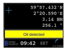
Unacknowledged alert is indicated as yellow background flashing and when alert is acknowledged yellow background stops flashing.
