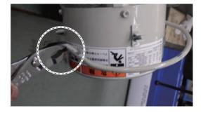
4. Remove the brake release lever pin with a pair of pliers.
