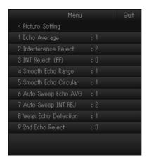
**[4 Smooth Echo RNG]**: Selects echo smoothing level in the range direction. The setting range is [0] to [5]. The higher the setting, the greater the smoothing.
