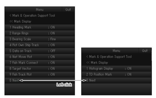
[1 Heading Mark]: The heading mark is a dashed line which indicates the heading in all presentation modes. It extends from own ship position to the outer edge of the display and appears at zero degrees in the head-up mode. Its orientation changes with ship's orientation in the north-up and course-up modes.
