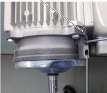
Check that the holes are aligned
