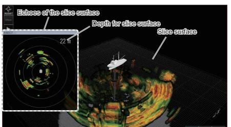
• [1 Cross-Section Movement] = [Scale-Based]: Shows the slices that are vertical to the sea surface.
