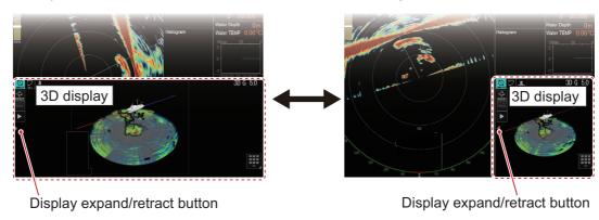
**Note 2:** You can change the 3D echo color according to echo strength or depth. To change the color reference, short-push the scrollwheel.
