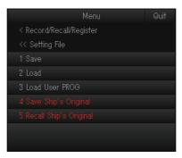
Left-click [1 Save]. The file name, which appears in the [File Name] box, is automatically assigned as shown below.
