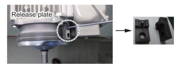
8. Referring to the following figure, unfasten the three screws, then remove the waterproofing cover and washer.
