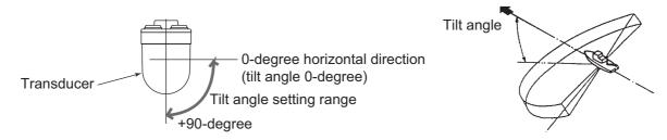
**Note 1:** In the sweep cross-section mode, the tilt angle is fixed at the angle set in the menu (see page 5-13).
