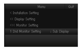
[1 2nd Monitor Setting]: When two monitors are used, select what to show on the sub monitor. Restart the system after changing this setting.
