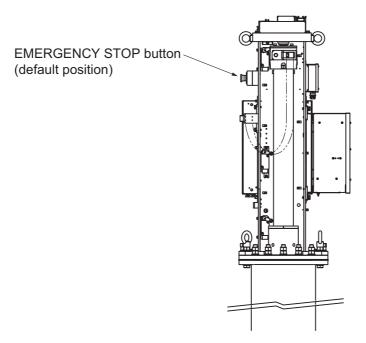
To release the emergency stop condition, first confirm that no one is near the hull unit. Then do the following:
