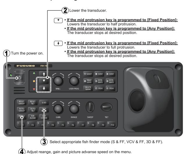
**Note:** In the default setting, slant (S) and vertical Slant (VCS) modes are active. To use other display modes, register the display mode to use from the menu. For how to register display modes, see section 1.6.2.
