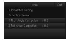
[1 Pitch Angle Correction]: Offsets the pitch angle at the motion sensor.
