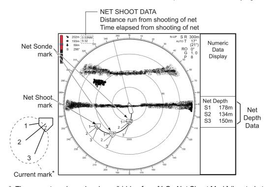
\*: The current mark can be shown/hidden from [4 On Net Shoot Mark] (located at main menu  $\rightarrow$  [0 Mark & Operation Support Tool]  $\rightarrow$  [6 Net Course Mark]). See section 9.2.6.
