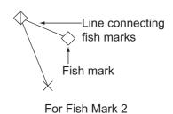
[8 Target Vector]: This is a line extending from the target lock mark, and it shows speed and direction of tracked school of fish. See the illustration at right for appearance.
