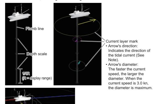
**Note:** Arrow's direction shows "from what direction the current is flowing" or "the direction the current is heading". [5 Current Flow Dir] on the [Current VEC & Wind]menu selects from what direction to display current data. See section 9.2.6.
