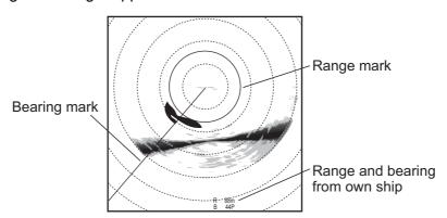
**Note 1:** You can clear the range and bearing marks and the indications at the bottom of the screen. Place the cursor on, or near, the own ship symbol, then press the **R/B AUDIO** key.
