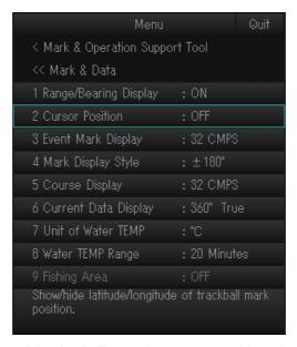
[1 Range/Bearing Display]: Turns the range and bearing data on or off.
