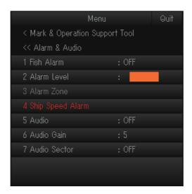
[1 Fish Alarm]: Turns the fish alarm function on or off. See section 2.15.1.
