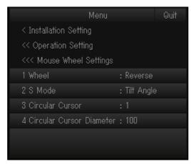
• [1 Wheel]: Sets setting value (detection range, gain, turn angle, user program number) increment direction.
