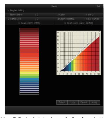
**[2 Signal Level]**: Contaminated water or reflections from plankton may be painted on the screen in green or light-blue. These echoes may be erased in order of strength. The setting range is [0] to [31]; [0] corresponds to the weakest color.
