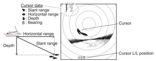
2. To measure the range and bearing to a different target, or mark the current target with its range and bearing, push the **R/B AUDIO** key. A range mark and bearing mark appear, intersecting the location selected at step 1. Further, the range and bearing to the target appear at the bottom of the screen.
