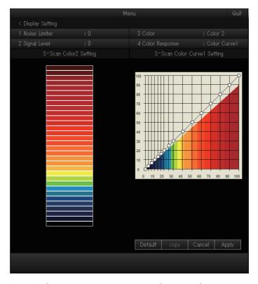
[2 Signal Level]: Contaminated water or reflections from plankton may be painted on the screen in green or light-blue. These echoes may be erased by strength. The setting range is [0] to [31]; [0] corresponds to the weakest color. Echoes weaker than the strength level set here are erased.
