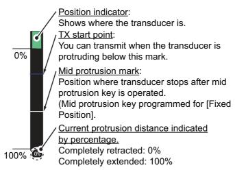
The color of the indicator changes according to transducer position and operation state.
