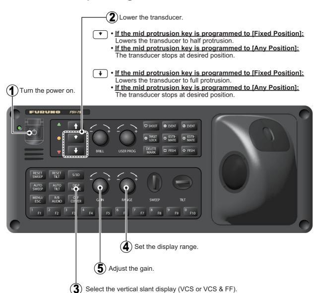
**Note:** In the default setting, slant (S) and vertical Slant (VCS) modes are active. To use other display modes, register the display mode to use from the menu. For how to register display modes, see section 1.6.2.
