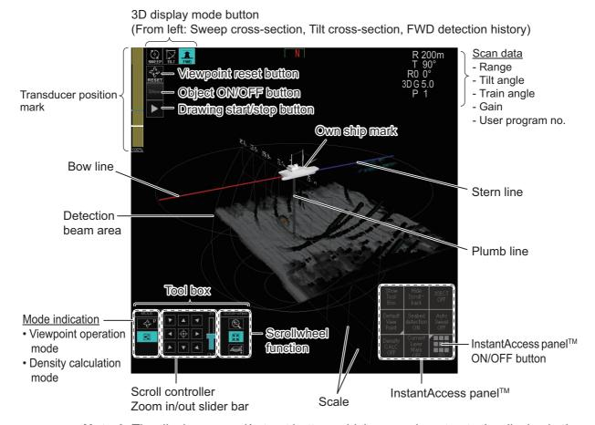
**Note 1:** The display expand/retract button, which expands, retracts the display in the 3D & S mode, is not shown in the default configuration. To show the button, [1 2nd Monitor Setting] on the [Monitor Setting] menu (see page 9-12) must be set to [Sub Display] or [OFF]. The button appears below the drawing start/stop button.
