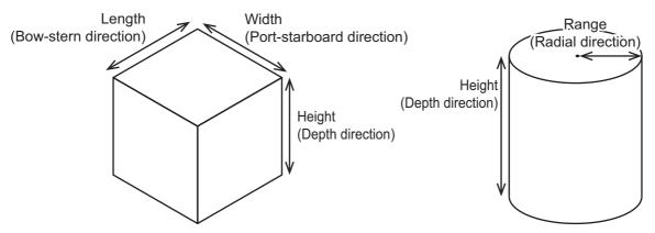
**For [Cylinder] measurements:** Adjust the values for [3 Height] and [4 Range] to adjust the calculation area size.
