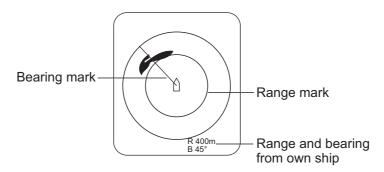
**Note 1:** You can clear the range and bearing marks and the indications at the bottom of the screen. Place the cursor on, or near, the own ship symbol, then press the **R/B AUDIO** key.
