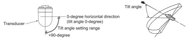
**Note 1:** The default function of the scrollwheel sets the tilt angle.
