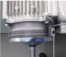
Check that the holes are aligned
