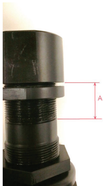
Figure 10. Gland nut travel measurement point for acetal and aluminium glands
