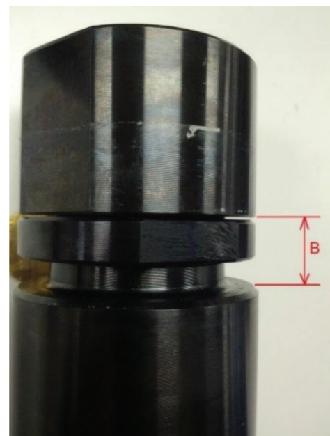
Figure 11. Gland nut travel measurement point for steel glands
