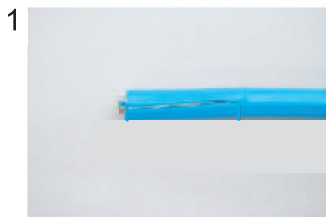
Expose inner vinyl sheath.
