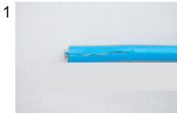
1 Expose inner vinyl sheath.
