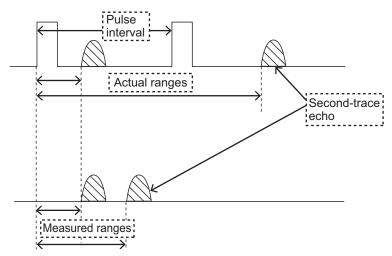
This equipment lengthens the pulse repetition period to reject false echoes.
