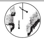
Relative target trails -Targets move relative to own ship, stationary targets are smeared.
