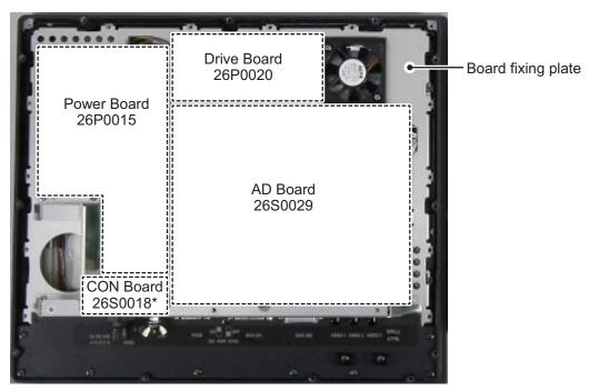
\*: CON Board 26S0018 is located under the overhang on the board fixing plate.
