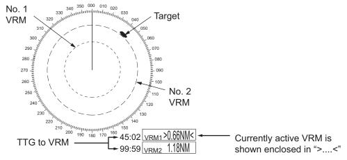
There are two methods for measuring range with the VRMs, using the **VRM** key and on-screen menu box operation.
