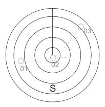
Place the cursor on a target, then press the **TGT ACQ** key to display the target data.
