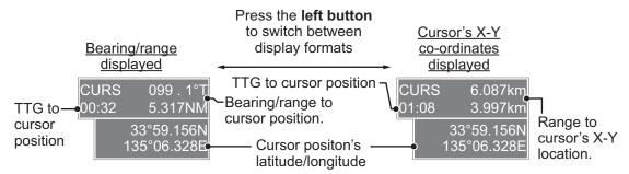
**Note 1:** For the X-Y co-ordinates display, the Y-axis is the heading line, the upper half of the screen is "plus" and the lower part of the screen is "minus". The X-axis is the port/starboard direction, starboard is "plus", port is "minus".
