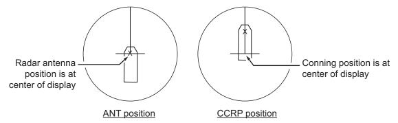
Range and bearing are measured and graphics are drawn according to reference position as in the table below.
