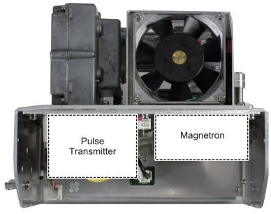
Transceiver module RTR-101 underside-rear view (For FAR-1518/1528/BB)
