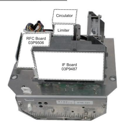
Remove IF Board 03P9487 to show MIC board 03P9505 (covered by board fixing panel).
