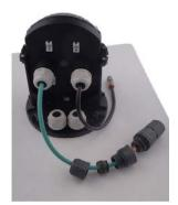
c. Remove the rubber boot from the end of the Ethernet cable using a cutter. It will not seal correctly with the rubber boot in place.
