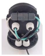
**b.** Wrap the tie around the groove in the corresponding end of the RJ45 coupler and tighten it to hold the coupler snugly against the back of the camera.
