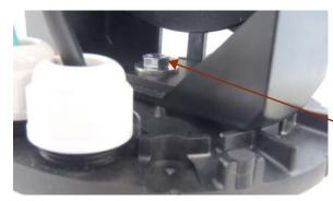
Loosen this bolt to adjust camera pan
