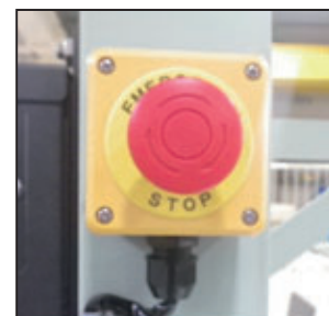
EMERGENCY STOP button
