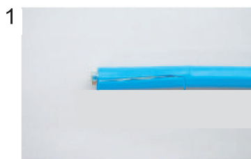
Expose inner vinyl sheath.
