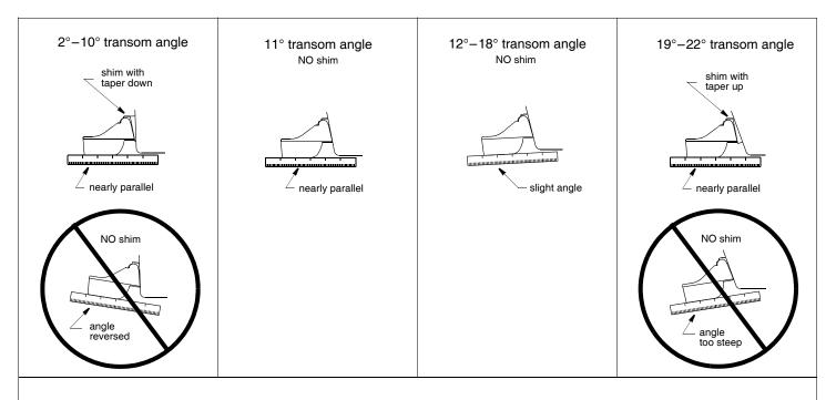
Figure 11. Sensor angle adjustment
