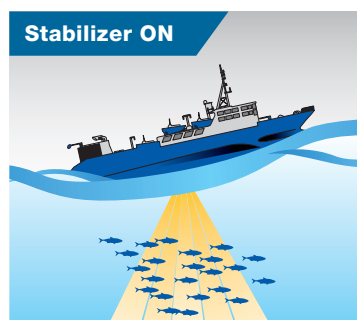
Stabilizer keeps the beam on the designated target.
