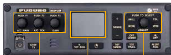
Rotate to adjust rain reflection, sea surface reflection, gain
